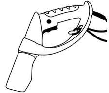
Fix the extension of the machine by inserting cable in the hook on the handle and plug onto the machine.
