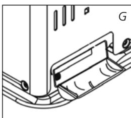
**4** Insert the batteries into their holder **11** at the back of the heater (Fig. G). Ensure that the positive and negative poles match the + and - marks indicated on the battery housing. Close the battery cover.
