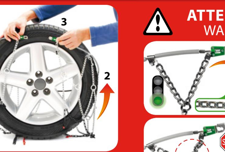
Recomendation, to wear high visibility jackets (signal color jackets) during mounting. Spread out the chain on the ground, with the yellow end of the cable to the left
