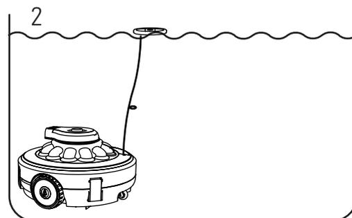
Adjust the length of the rope to ensure that the length of the rope is at the same height as the water level, and the extra length of the rope is tied or cut short.
