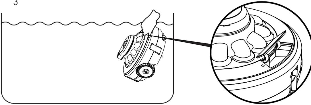
Adjust the length of the rope to ensure that the length of the rope is at the same height as the water level, and the extra length of the rope is tied or cut short.
