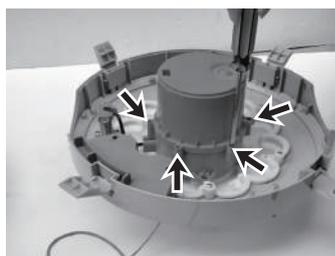
2. Use a screwdriver to remove all screws on the power cover of the bottom cover.
