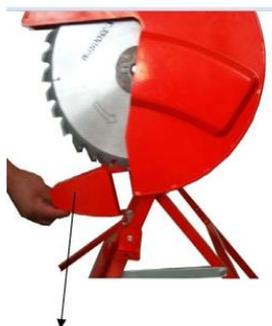
Disassemble the lower guard first
