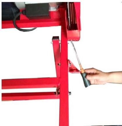
Connect the lower guard to the outer blade cover at the bottom. Tighten them with 2 bolts (M6x12) and 2 flat washers ( $\text{Ø}6$ )
