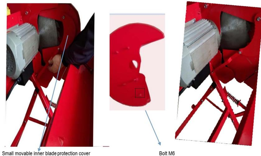
Fix the small movable inner protection cover to the outer blade cover by putting it into the bolt M6 at the bottom of the outer blade cover. Then tighten it by 1 locking nut (M6).
