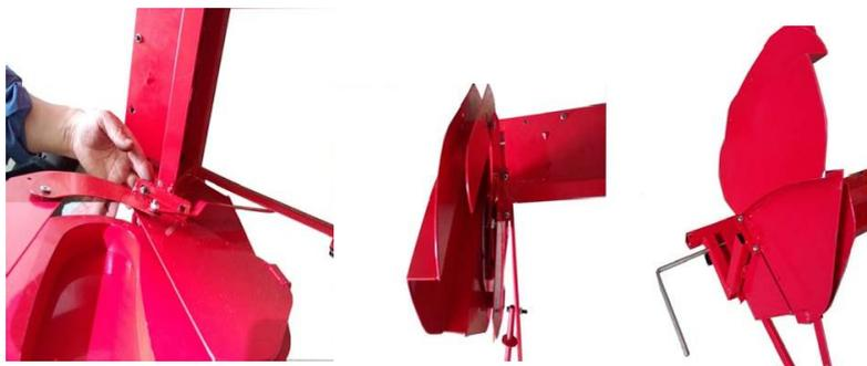
Connect the inner blade cover and the work table by putting 4 bolts (6x15) into the hole on the work table plate. Then tighten them by 4 flat washers ( $\varnothing 6$ ) and 4 locking nut (M6).
