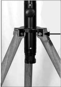
1. Insert the three tripod legs into the holes of the tripod leg holder, insert the 3 screws for each leg and tighten the nuts.
