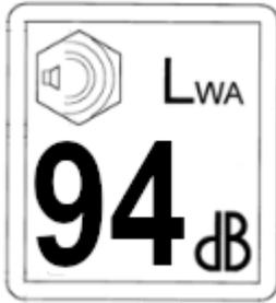
Calculation of the measured and guaranteed sound power level was carried out according to the procedure in Directive 2000/14/EC, Annex V.
