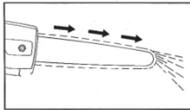
If there are no traces of oil, check to have refilled the tank.
