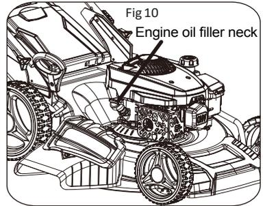
**⚠ CAUTION** To prevent engine damage the engine is shipped without oil or petrol. The engine must be filled with the correct grade of oil and petrol before starting the engine.
