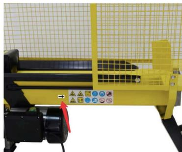
Before operating the log splitter, the Bleed Screw should be loosened by some rotations until air can go in and out of the oil tank smoothly.
