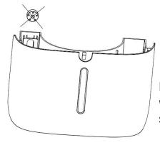
If the tank is dirty, clean it with cold or warm water. Do not use detergent, stee wool, chemical dust removal cloth, gasoline, benzene, diluent or other solvents, because it may damage the water tank and cause water leakage.
