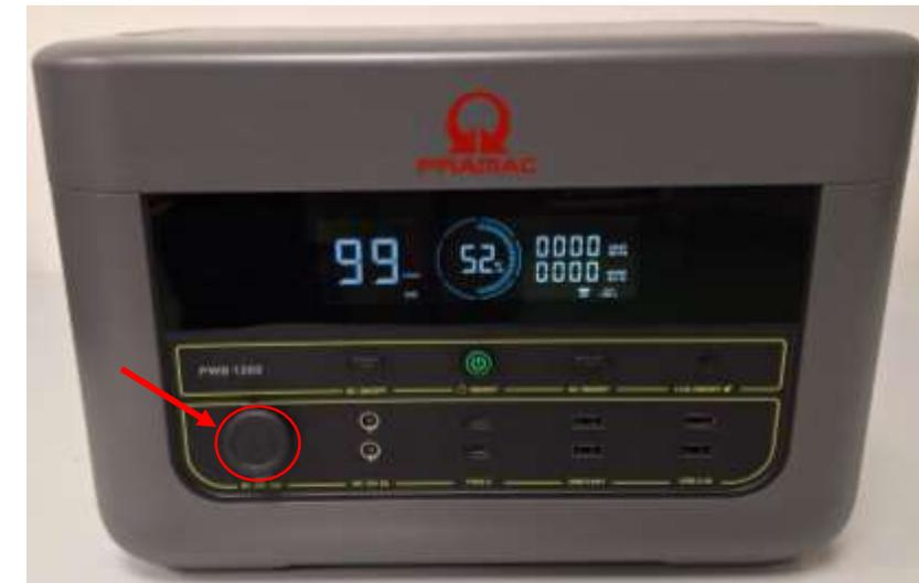
4. DC switch, press this button to activate the 12V DC outputs.
