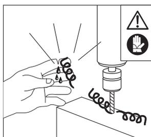
Sharp and hot chips which cause cuts and burns to the hands and body. Wear protective gloves and use a hook to remove chips.
