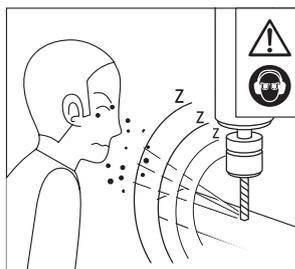
Material flying towards the operator's eyes and body. Loud noise. Wear eye protection goggles and ensure the cutting area is positioned correctly. Use ear protection.
