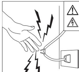
Risk of electric shock and danger of death. Do not touch live electrical parts and keep a safe distance. Before any maintenance disconnect the plug from the power outlet.
