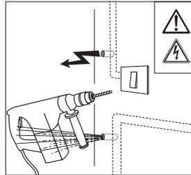
Risk of electric shock or explosion due to puncture of electrical conduits or pipes containing pressurized fluids (water, gas ... ) . Hold with both hands 2 insulated
