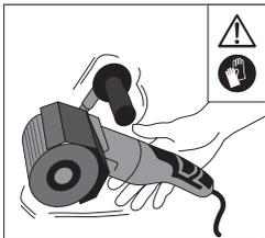
Danger of high vibrations. Put on anti-vibration gloves. Take rest breaks while working.
