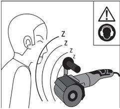
High noise generated during machining. Wear hearing protection headphones.
