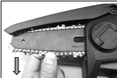
3. Turn the lever clockwise until the sprocket cover is secured then return it to the original position.
