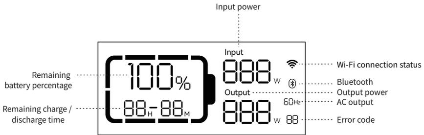
**Battery capacity:** When power station is being charged, SOC icon will flicker.
