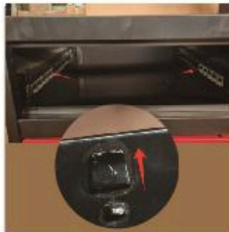
Step 10: Assemble P rail for 6 drawers. Note the slip must upward
